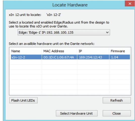
The Locate Hardware dialog will scan the selected Radius, Prism, or Edge unit and list xIn or xOut 12 units. Select the physical xIn or xOut 12 unit you wish to use and click the Select Hardware Unit button.
