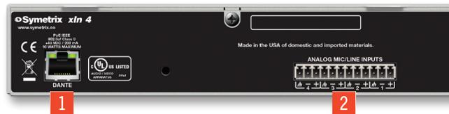
**1 Dante (Primary):** 100 Base-T Ethernet port provides 8 (4x4) channels of Dante network audio, Ethernet communications, and power.
