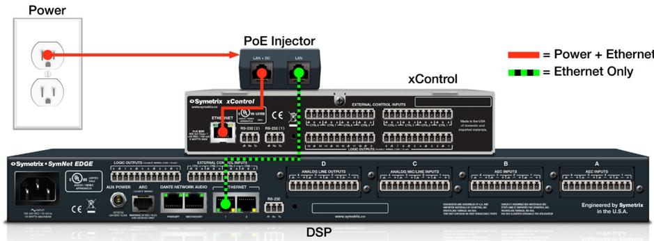
Direct connection to DSP using PoE injector.
