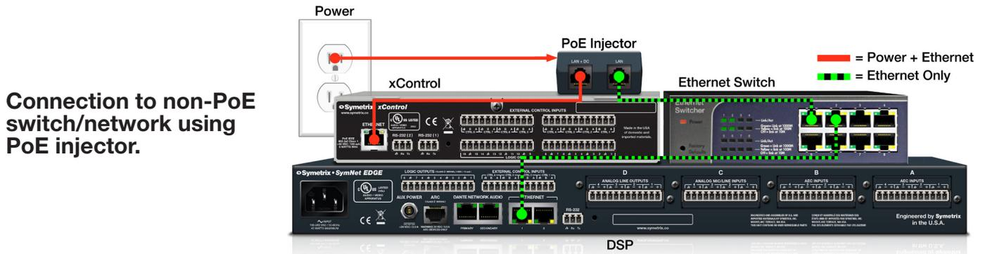
Connection to non-PoE switch/network using PoE injector.
