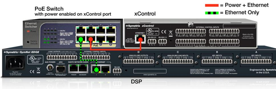
Connection to PoE switch/network without PoE injector.
