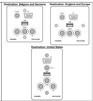
The WAV-6UBA is a one gang wall plate insert that has one USB connector (type B) at the front and a cable with a USB connector (type A) connector at the rear. In addition, the WAV-6UBA has pass through connectors for:
