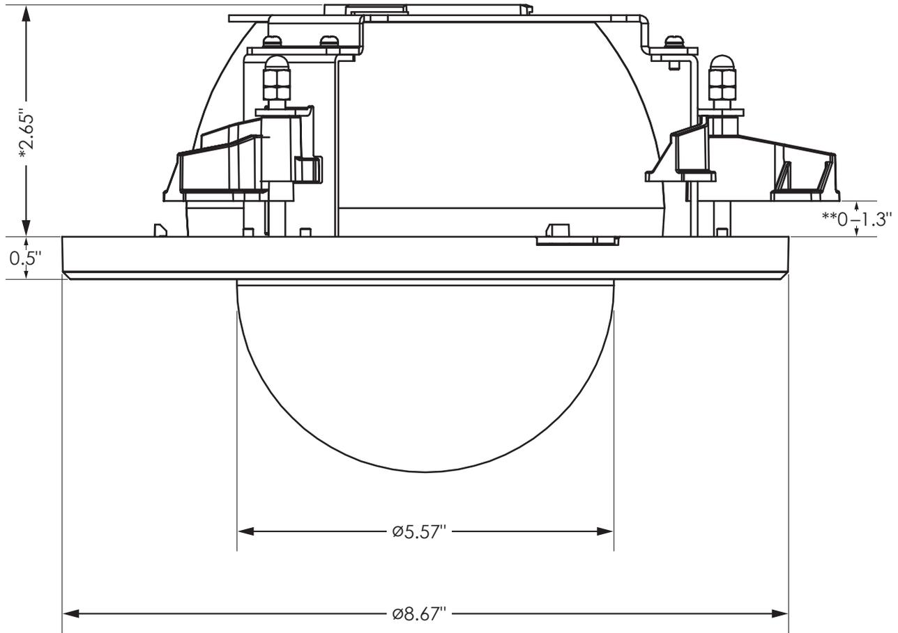
\* Dimension includes height of camera installed in the bracket.
