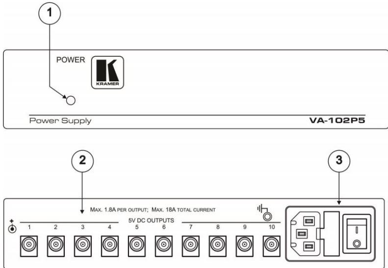
Figure 2: VA-102P5 10-Output 5V DC Power Supply
