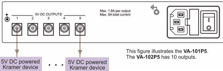
This figure illustrates the VA-101P5. The VA-102P5 has 10 outputs.
