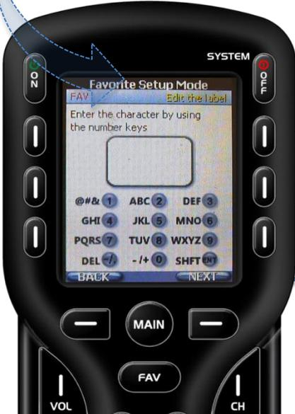
Enter the **channel name** using the alphanumeric keypad.
