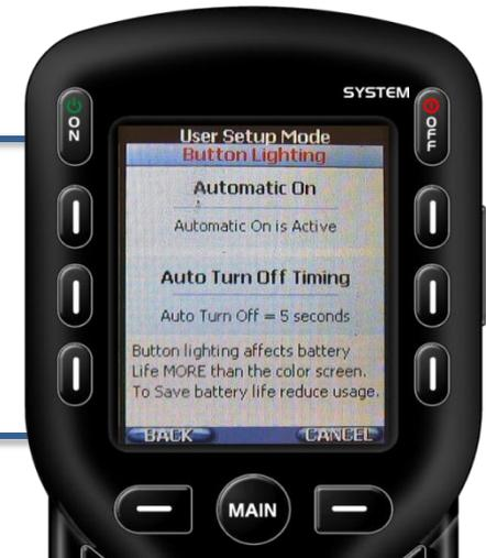
**Automatic On:** ON when LCD is ON, or Always OFF
