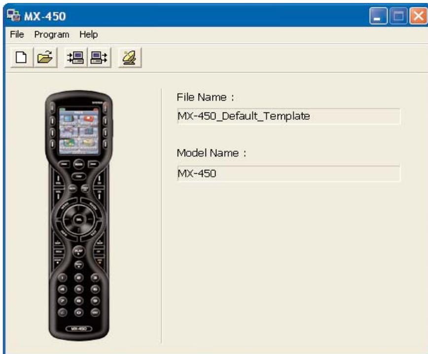
The MX-450 Archiver is designed to enable the professional installer to archive configurations programmed on either the MX-450 remote control so that the configurations can be reused in the future without repeating the programming process. Downloading a previously programmed configuration often provides a better starting point for programming and speeds customization even if the new system is slightly different from an archived file.
