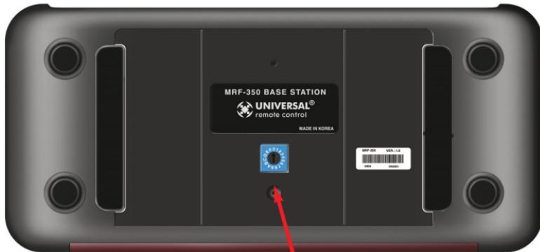
Slide off the mounting plate to reveal the RF ID# rotary switch. Check that the arrow pointer in the center of the wheel is pointed to 0, the default “interference sniffing” position. If it is not, use a small flat blade screwdriver (included) to set the RF ID# to 0.
