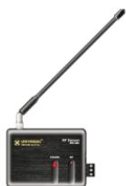
When testing, set both the remote and the MRF-350 to the same VALID RF ID#. Keep in mind that zero (0) is not a valid RF ID#. Watch the STATUS LED on MRF-350 - it should light every time you press a button on the remote. This will tell you that the signal was received and understood. You can ignore the RF LED on the RFX-250 (it only indicates that a signal was received, not that it was understood).
