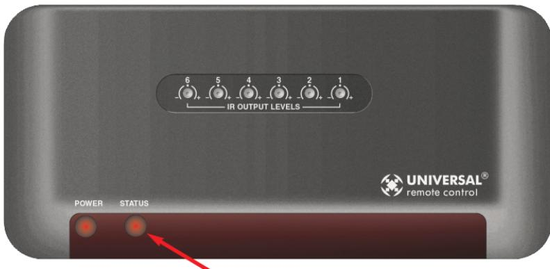
The flickering or glowing STATUS LED warns you that the RFX-250 is detecting RF interference generated or reflected near this location. MOVE the RFX-250 to a new location.
