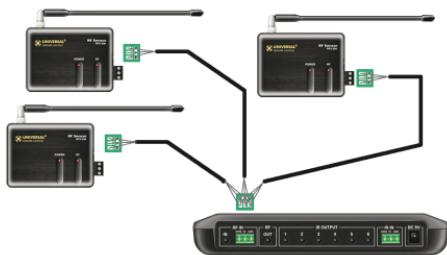
9. Should you need more than six IR Outputs, connect as many as three different MRF-350s to one RFX-250 in a daisy chain using the supplied cable.
