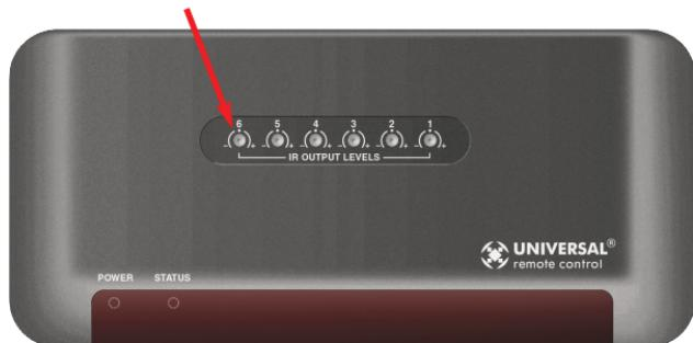
**NOTE:** TiVo, Replay TV, Satellite Receivers and Cable Boxes are all extremely sensitive to IR overload or saturation. Put up the on screen guide and test the navigation arrows. Compare operation via RF to the original remote control. Operation should be identical. RF is not slower. If operation is inconsistent or sluggish, LOWER the IR line output.
