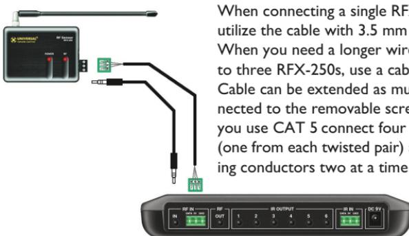
When connecting a single RFX-250 to the MRF-350 utilize the cable with 3.5 mm plugs on both ends. When you need a longer wire or are connecting up to three RFX-250s, use a cable with tinned ends. Cable can be extended as much as 200', then connected to the removable screw connector plugs. If you use CAT 5 connect four conductors to GND (one from each twisted pair) and connect the remaining conductors two at a time to 5V and DATA .
