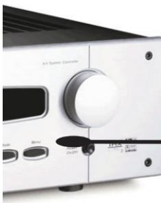
4. Self-adhesive “Flashers” affix to the Infrared sensors on the front panels of your client's components. The Flashers relay commands to components out of sight of the MRF-350's Front Blaster. The flashers plug in to the MRF-350's rear flasher line outputs via their 10 foot cables. Uniquely, the MRF-350 can also connect to rear panel IR Inputs via its adjustable IR Line Outputs.
