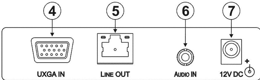
Figure 2: TP-121xl UXGA/Audio Line Transmitter Rear Panel
