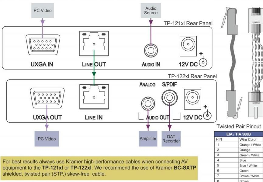
For best results always use Kramer high-performance cables when connecting AV equipment to the **TP-121xl** or **TP-122xl**. We recommend the use of Kramer **BC-SXTP** shielded, twisted pair (STP), skew-free cable.
