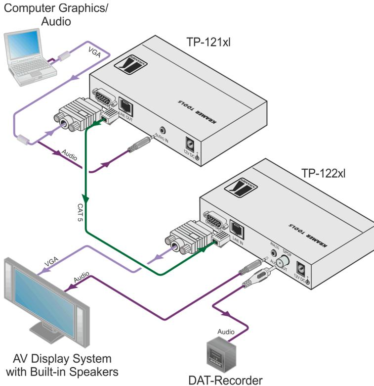
Figure 5: Connecting the TP-121xl Transmitter and TP-122xl Receiver
