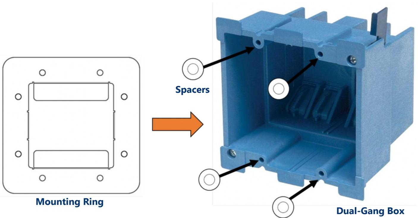
Use the spacers as a buffer between the mounting ring and dual-gang box, this can be done by using a screw to secure the mounting ring and spacers to the box.
