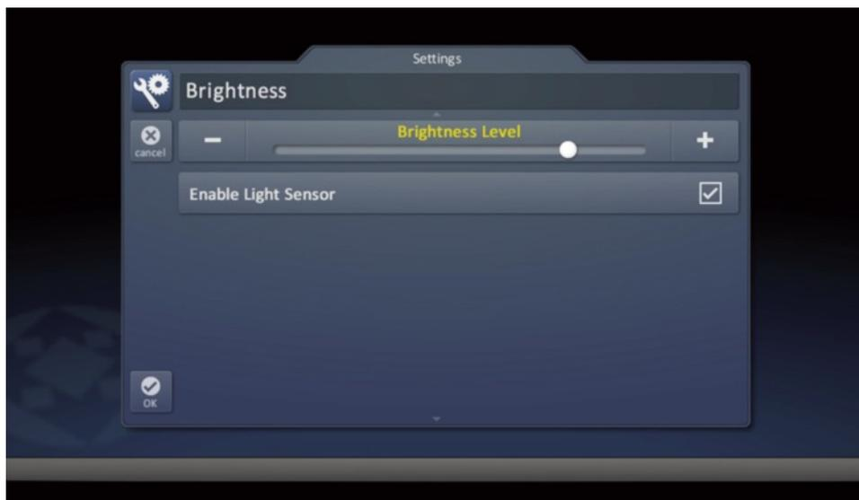
Selecting **Enable Light Sensor** disables the **Brightness Level** selection and dynamically adjust the LCD brightness based upon the ambient room lighting detected by the light sensor.
