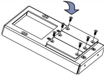
Mount the inner frame into the **TBUS-5xl** enclosure.
