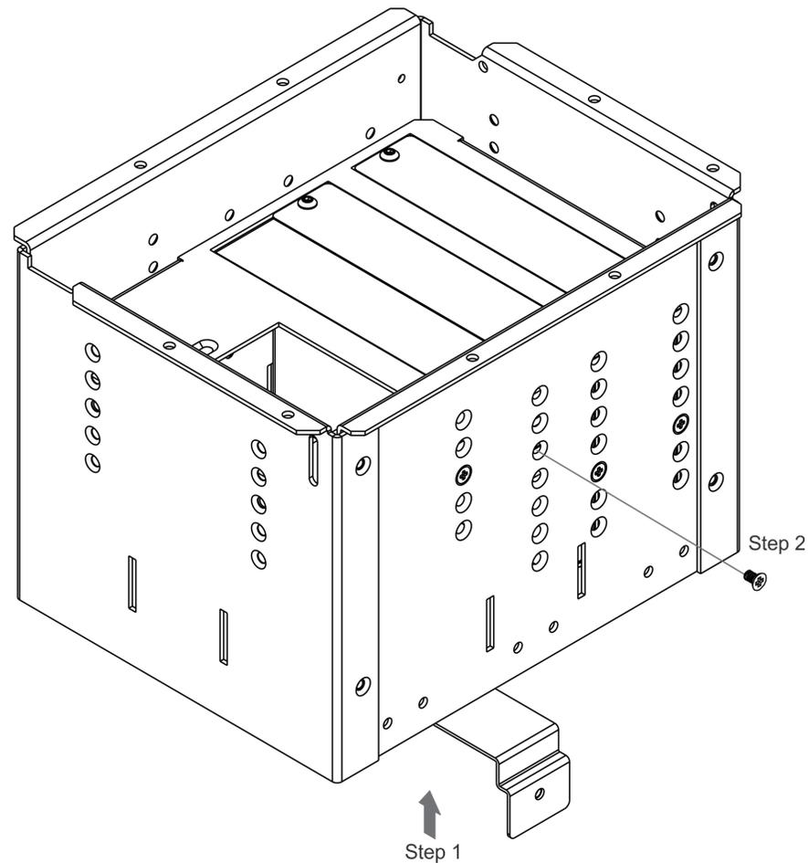
Figure 2: Installing the T-TBLANK TOOL Blank
