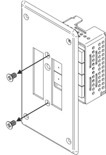
Figure 2: RC-8IR Faceplate Holes Insert Kit for RC-8IR
