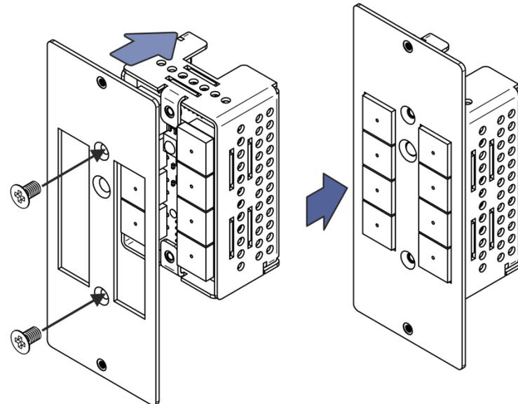
Figure 3: T-RC-8IR Installation
