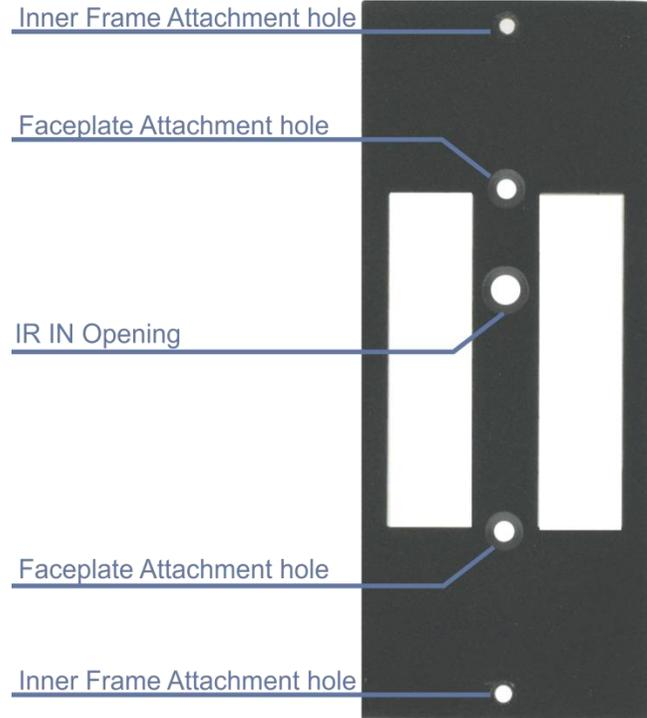
Figure 1: T-RC-8IR Insert Kit for RC-8IR (P/N: 80-000599)
