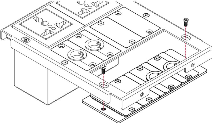
Figure 2: T-4INSERT Installation, Step 1
