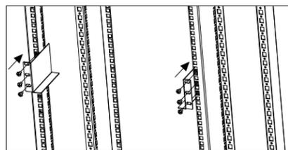
Attach support brackets at the back of the rack.
