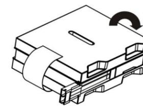
Place the cover back on the battery tray and reassemble the UPS.
