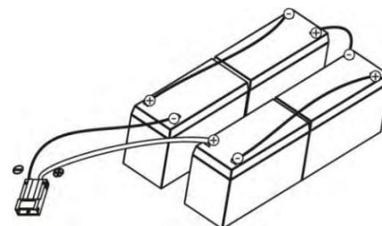
Replace the batteries in the tray. Wire the new batteries as shown above.
