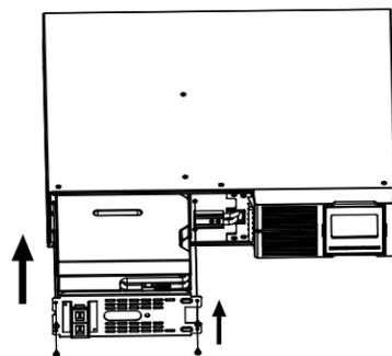
After swapping the batteries, replace the battery tray in the UPS and reattach the battery cover. Tighten the screws securely.
