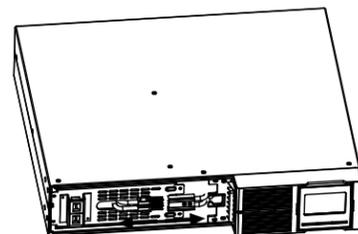
Disconnect the battery wires.
