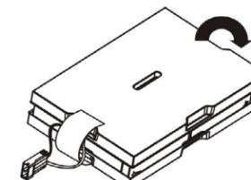
Place the cover back on the battery tray and reassemble the UPS.
