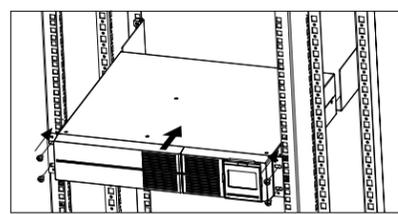
Mount the UPS in the rack with the rear of the unit resting on the back brackets.
