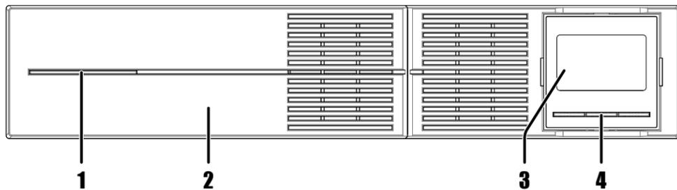
1. Power LED – Illuminates solid blue when the UPS is powered on.
