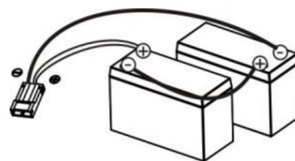
Replace the batteries in the tray. Wire the new batteries as shown above.
