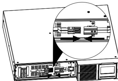
Connect the battery wires.
