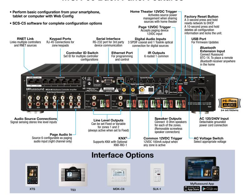
The Russound MCA-66 digital multi-zone controller amplifier provides up to six zones of distributed audio, for up to 6 audio sources. Scalable to 36 zones, the MCA-66 provides numerous options to tailor to residential or light commercial distributed audio systems. The Bluetooth® connection allows the installation of the MCA-66 in an equipment rack while remotely locating the optional Russound BTC-1X Bluetooth receiver up to 300' away. Additionally, the BTC-1X improves audio quality through
