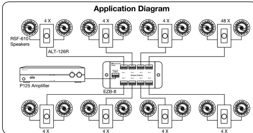
The application diagram above shows an EZB-8 being used to run 8 pairs of Russound RSF-610 speakers using 8 ALT-126R volume controls, with each volume control's impedance switch set at the 4X position. The speakers are wired to their volume controls and the volume control wires run back to the EZB-8 where all 8 pairs of wires are easily connected to the EZB-8. The P125 amplifier is then connected to the EZB-8 connector marked "Input from Amplifier"
