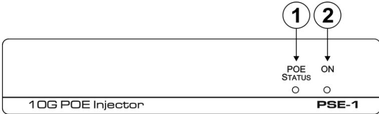
Figure 1: PSE-1 10G POE Injector Front Panel
