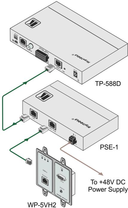
Figure 3: Connecting the PSE-1 10G POE Injector
