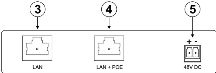
Figure 2: PSE-1 10G POE Injector Rear Panel
