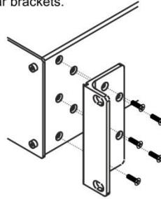
2. Place the ears of the machine against the rack rails, and insert the proper screws (not provided) through each of the four holes in the rack ears.
