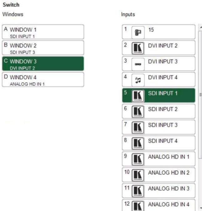
Figure 20: Switching an Input to a Window
