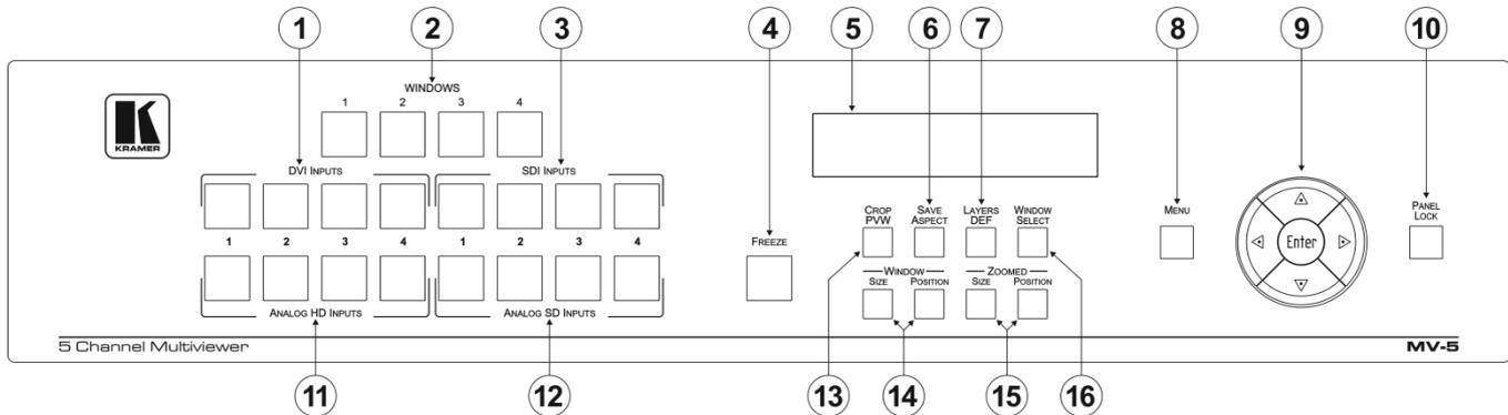
Figure 1: MV-5 5 Channel Multiviewer Front Panel
