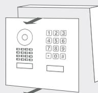
Pull the front panel with attached Main Electrical Unit out of the mounting housing (backbox).
