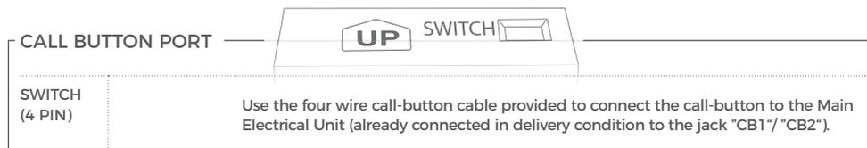
**NOTICE** Please take care when connecting the cables and wires. Connecting the cables and wires the wrong way may damage the device. Wires without insulation material must not protrude out of the green screw connection terminal, it may lead to electrical short and damage the device.
