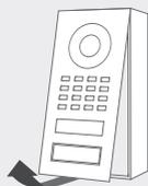
Pull the front panel with attached Main Electrical Unit out of the mounting housing (backbox).
