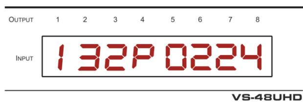
In this example: Input 1 is routed to output 1, input 3 is routed to output 2, input 2 is routed to outputs 3, 6 and 7, a pattern is routed to output 4, output 5 is set to mute, and so on.
