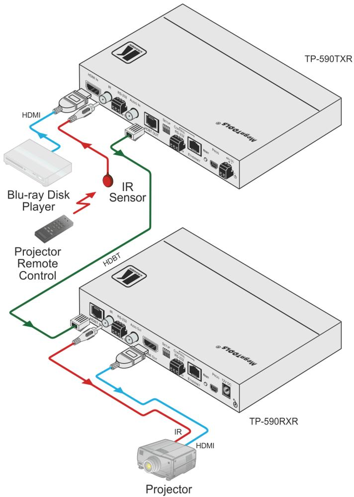
Figure 5: Controlling a Projector via the TP-590Txr
