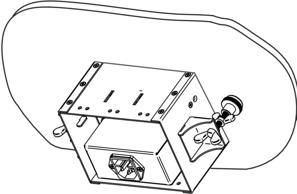
Figure 5: Locking TBUS-3US-22 under the Table
