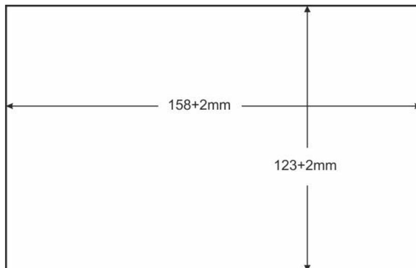
Figure 3: Cut-out Dimensions (not to scale)
