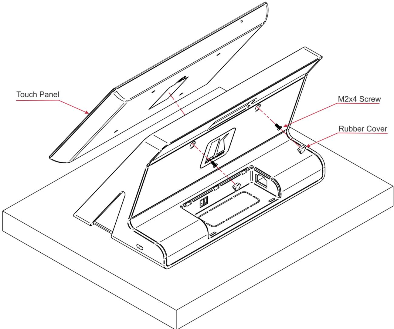
Figure 9: Connecting to the KT-107 Rear Panel
