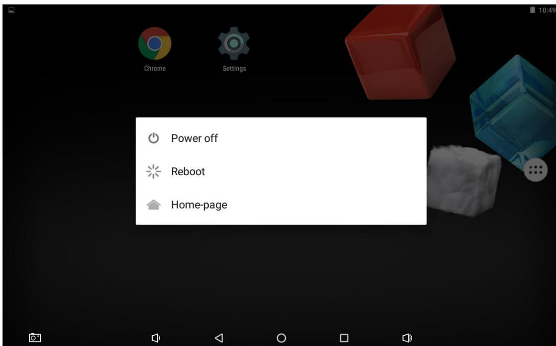
Figure 32: Using a Hidden Control Button
