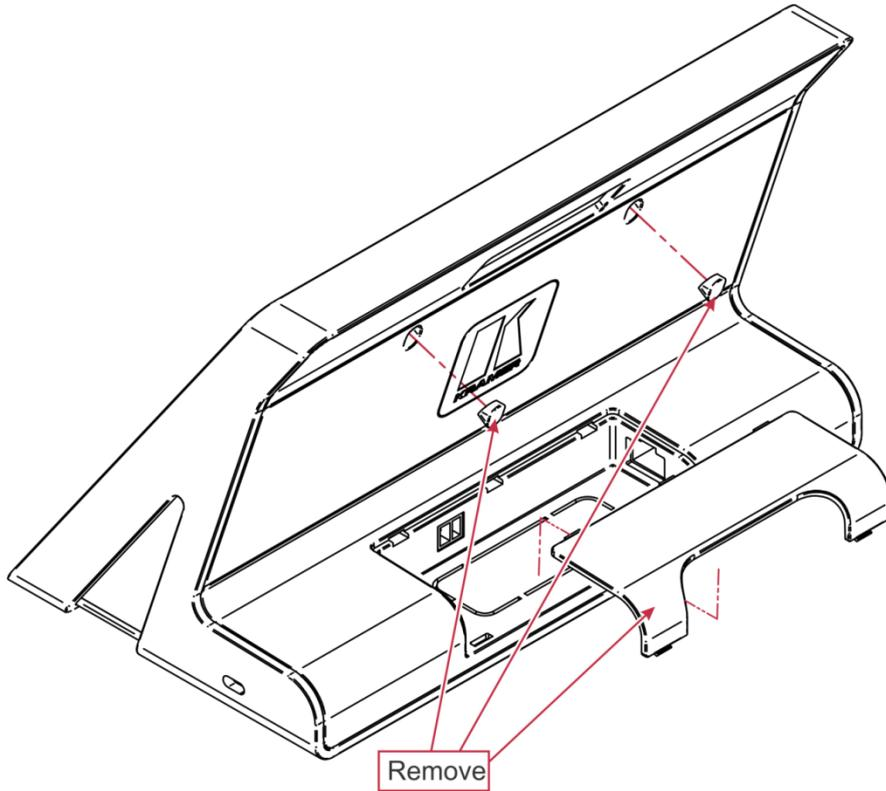
Figure 7: Removing Cable Cover and Rubber Screw Cover
