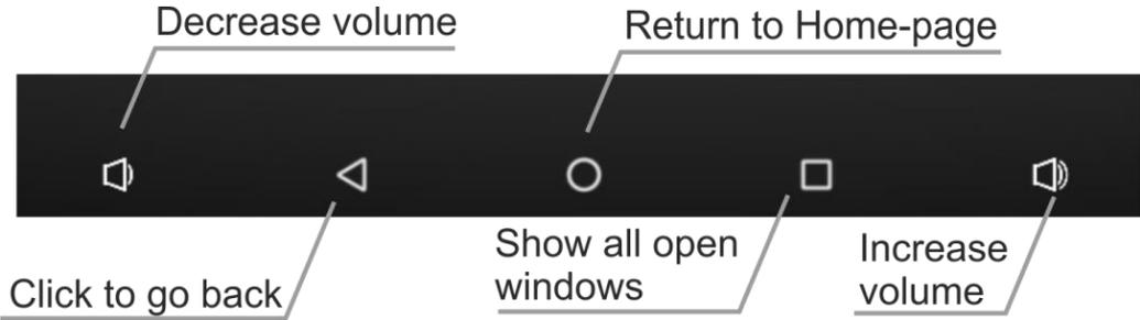
Figure 37: KT-107 Lower Bar Functions
