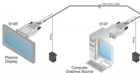
Always use Kramer high-performance cables for connecting AV equipment to the **614T/R**.
