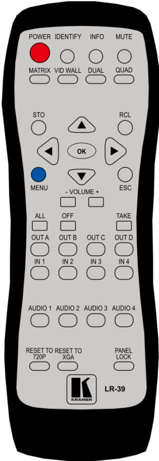
Figure 18: Infrared Remote Control Transmitter
