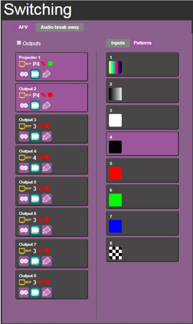
Figure 31: Switching Page – Switching a Pattern to an Output
