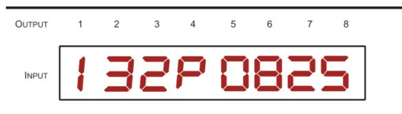
In this example: Input 1 is routed to output 1, input 3 is routed to output 2, input 2 is routed to outputs 3 and 7, a pattern is routed to output 4, output 5 is set to mute, and so on.
