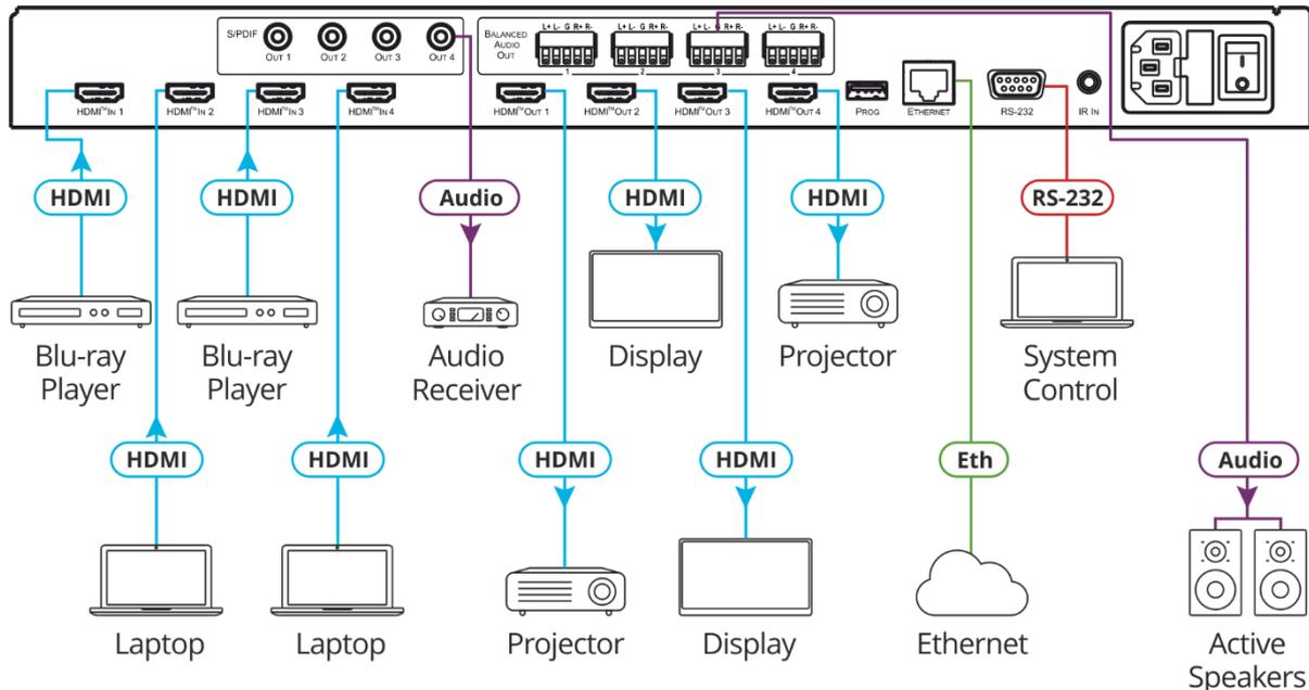
Figure 3: Connecting to the VS-44H2A Rear Panel
