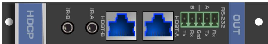
The **HDBT7-IN2-F16** and **HDBT7-OUT2-F16** cards feature Kramer Equalization and re-Klocking™ technology. The cards include a 3.5mm jack for connecting an IR emitter, such as the **C-A35M/IRE**, or an IR receiver, such as the **C-A35M/IRRN**. The **HDBT7-IN2-F16** and **HDBT7-OUT2-F16** cards also include a terminal block for connecting via RS-232. For information on connecting via RS-232, see [Connecting to the VS-1616DN-EM via RS-232](#) on page [13](#).
