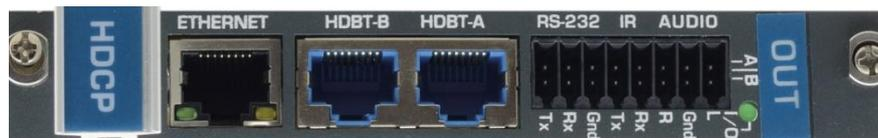
The **DTAxr-IN2-F16** and **DTAxr-OUT2-F16** cards include a terminal block for connecting analog audio, RS-232, an IR emitter, such as the **C-A35M/IRE**, or an IR receiver, such as the **C-A35M/IRRN**. For information on the IR wiring scheme, see [IR Wiring Scheme for HDBT Cards](#) on page [53](#). For information on connecting via RS-232, see [Connecting to the VS-1616DN-EM via RS-232](#) on page [13](#).
