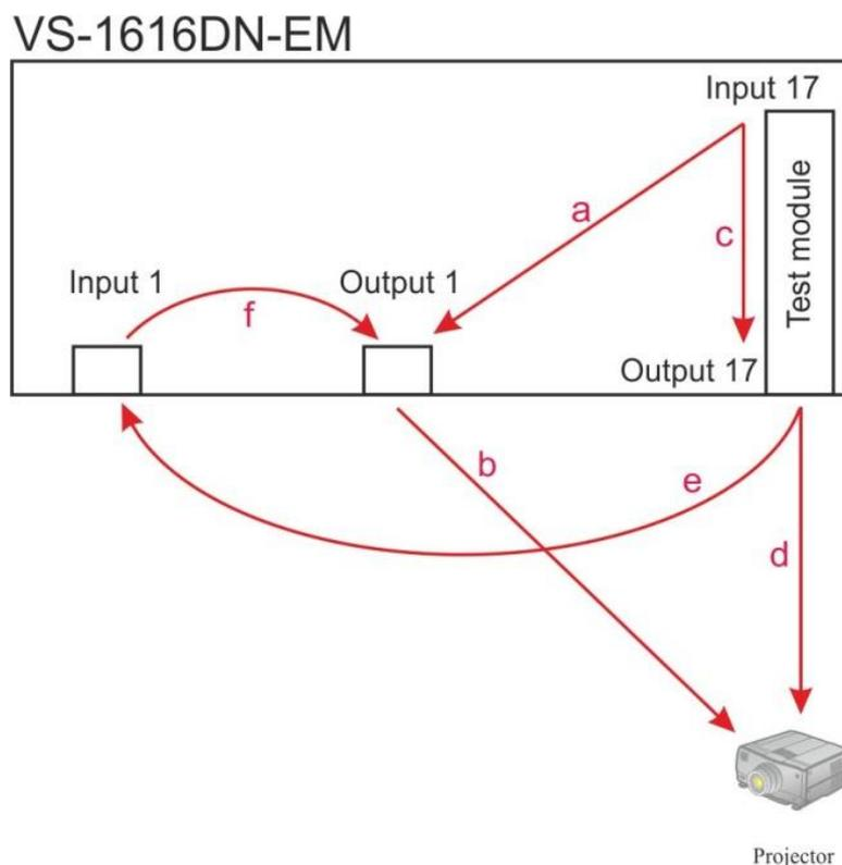
Figure 16: Signal Paths for Isolating Video Problems
