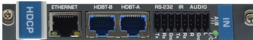
The **DTAxr-OUT2-F16** is a 2-output 4K60 4:2:0 HDMI over HDBaseT card with selectable embedded or de-embedded analog audio (F-16). The **DTAxr-OUT2-F16** outputs two extended reach HDBaseT signals with analog audio, bidirectional RS-232, and IR from the chassis to the line.
