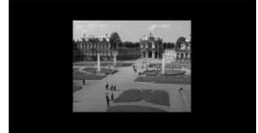
**FOLLOW OUTPUT** – The aspect ratio and resolution of the input signal is re-sized to precisely match the aspect ratio and resolution of the **VP-778** output signal. This may result in some distortion to the input signal images.
