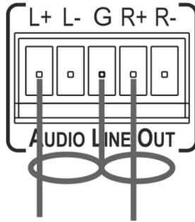
Figure 10: Connecting an Unbalanced Stereo Audio Acceptor to the Balanced Output
