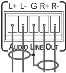
Figure 9: Connecting the Balanced Stereo Audio Output
