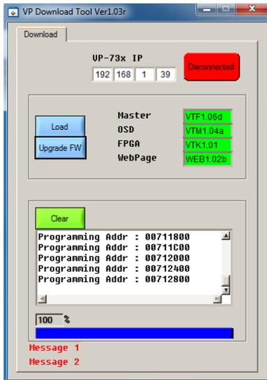
Figure 23: Firmware Upgrade – the VP Download Tool
