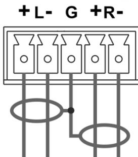
Figure 4: Connecting the Balanced Stereo Audio Output
