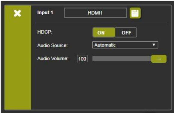
Figure 14: Setting Window for Input 1
