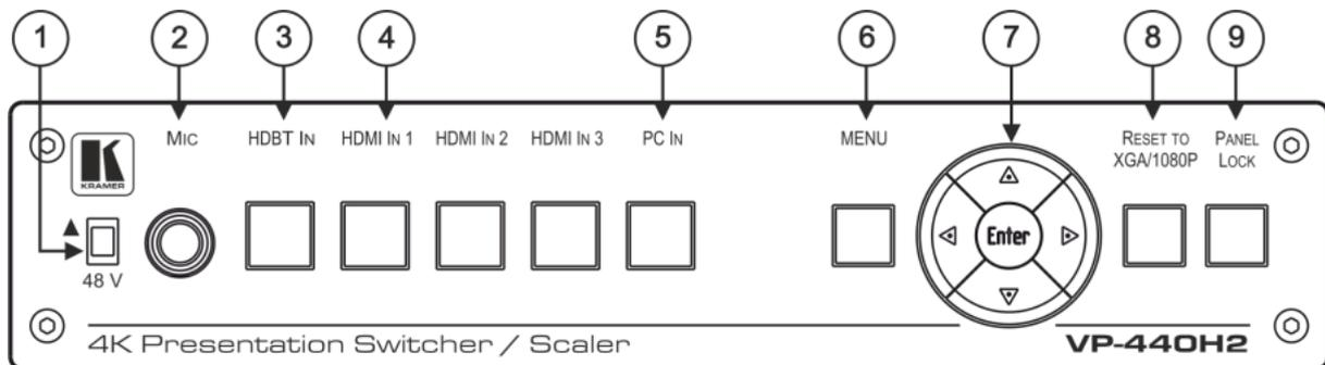
Figure 1: VP-440H2 4K Presentation Switcher/Scaler Front Panel
