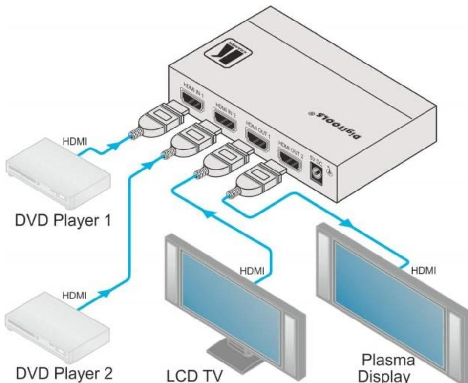
Figure 2: Connecting the **VM-22H** 2x1:2 HDMI Switcher/DA
