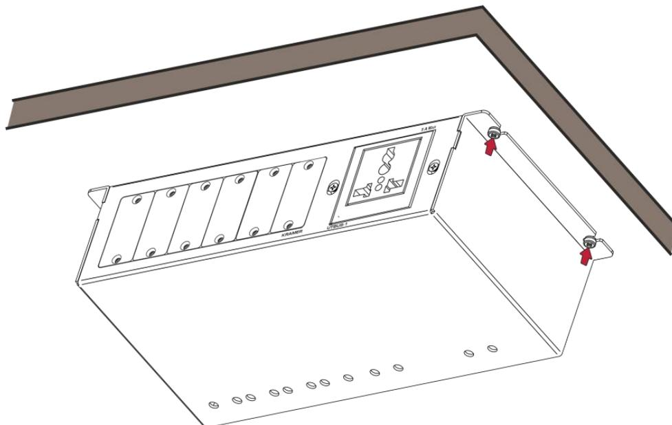
Figure 4: Securing the UTBUS-1xl Under the Table
