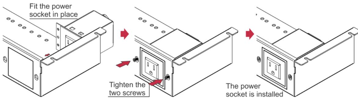
Figure 3: Installing the Power Socket
