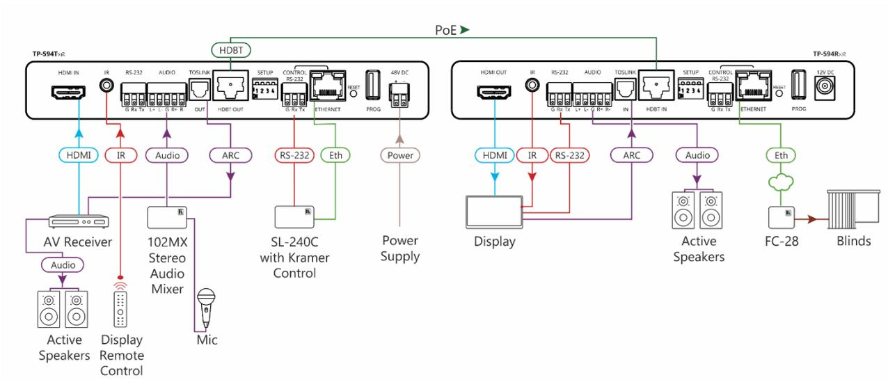
Figure 3: Connecting to the TP-594Txr Rear Panel
