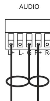
Figure 5: Connecting to an Unbalanced Stereo Audio Acceptor
