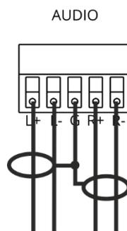
Figure 4: Connecting to a Balanced Stereo Audio Acceptor
