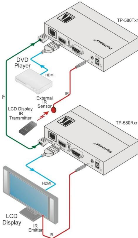
Figure 5: Controlling an LCD Display via the TP-580Txr
