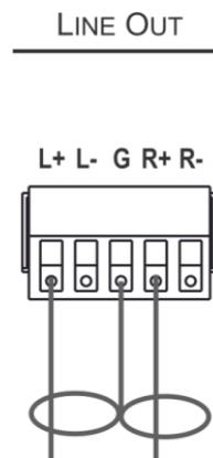
Figure 4: Connecting to an Unbalanced Stereo Audio Acceptor
