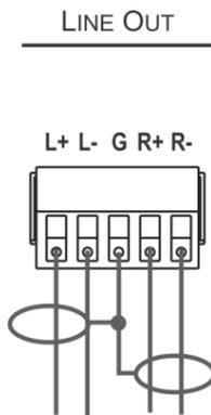
Figure 5: Connecting to a Balanced Stereo Audio Acceptor
