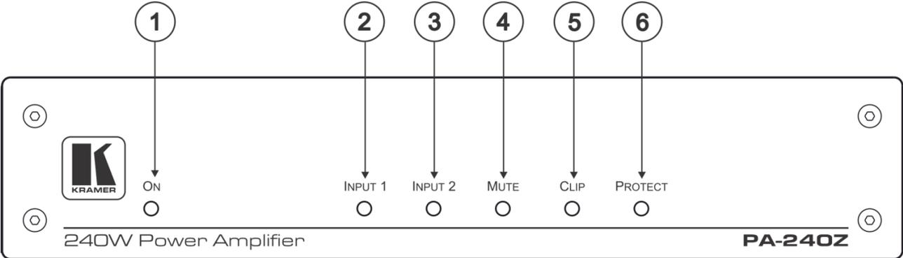
Figure 1: PA-240Z 240W Power Amplifier Front Panel
