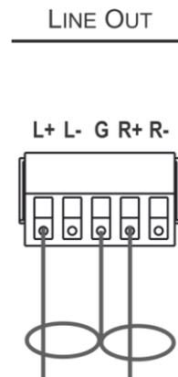
Figure 6: Connecting to an Unbalanced Stereo Audio Acceptor
