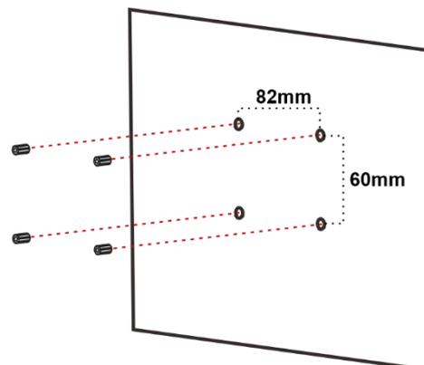
4. Attach the wall bracket to the wall, using the four wall-bracket screws.
