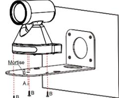
5. Attach the device to the wall bracket by fitting the mortise (on the bracket) into the tenon (on the camera).
