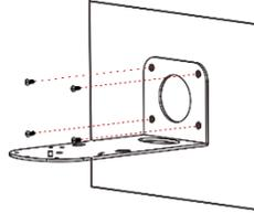
4. Attach the wall bracket to the wall, using the four wall-bracket screws.
