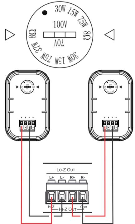
The following diagram displays the Galil 6-AW speakers connected to a recommended Kramer power amplifier (for example, PA-120Z):
