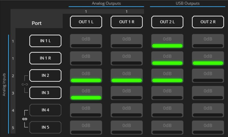
Figure 37: Matrix Page – Multiple Input-Output Cross-Points
