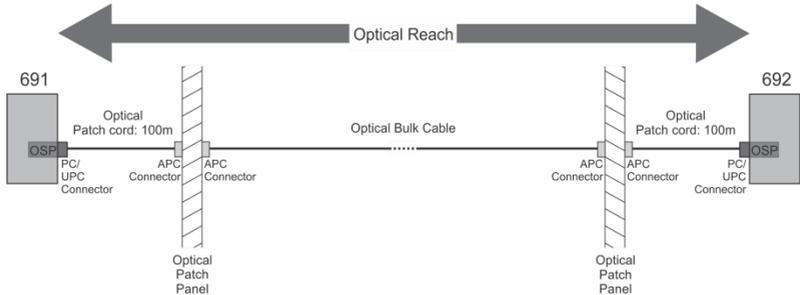
Figure 5: System Layout Example for Optical Reach Evaluation
