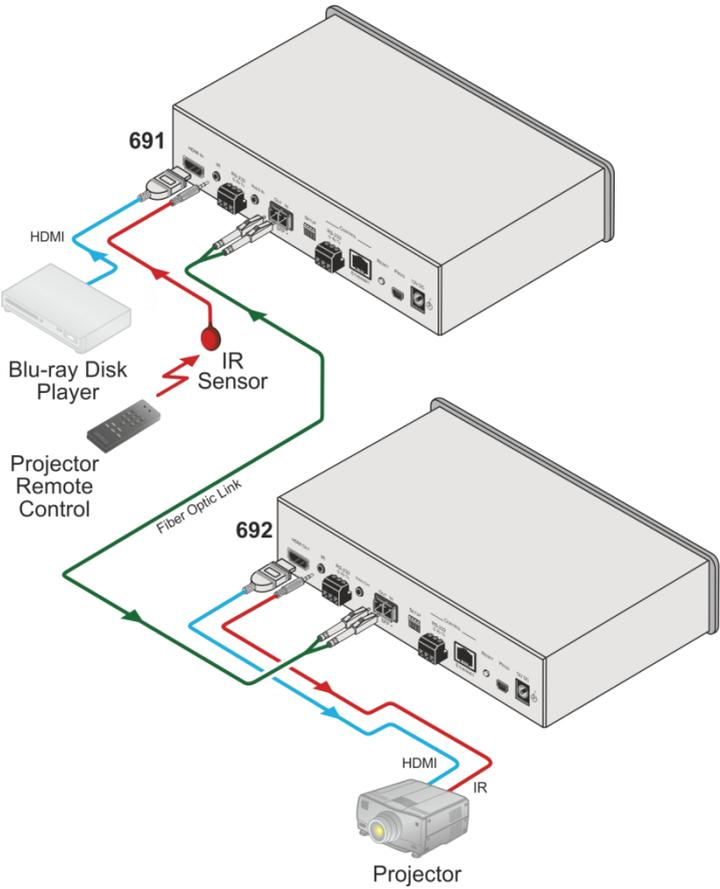
Figure 13: Controlling a Projector via the 691 Transmitter
