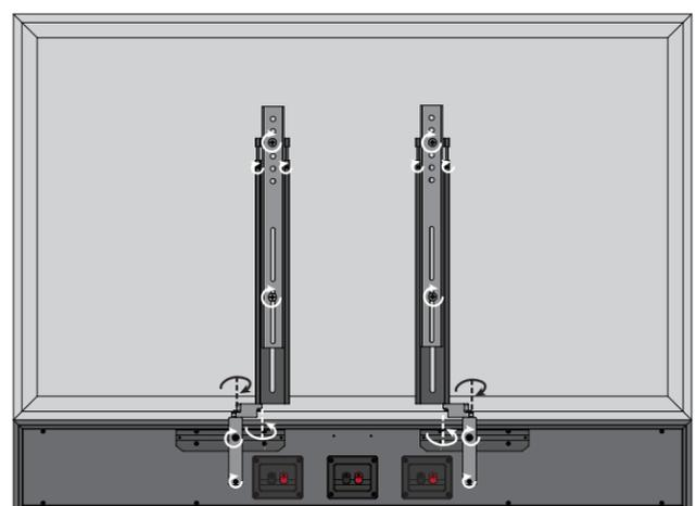
Tighten all screws and set screws down before mounting and wiring the TV and speaker. 2 people are needed for this task.
