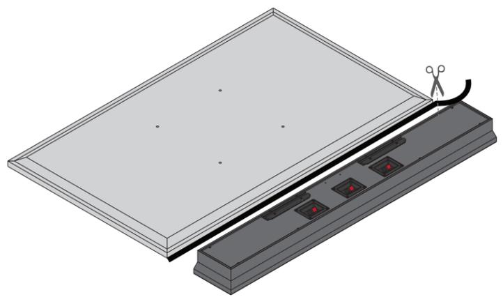
{Optional} For TVs with clear bezels or gaps between speaker and TV, apply **Foam Tape** to TV's edge and cut to size.
