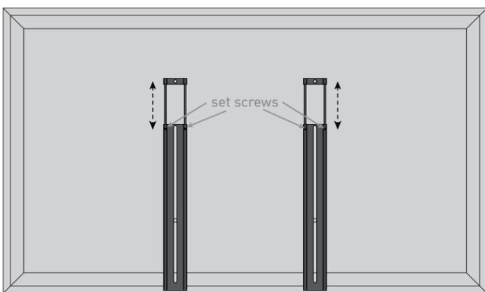
Loosen set screws on **Adjustable Uprights**. Slide **Adjustable Uprights** to align with TV mount holes.
