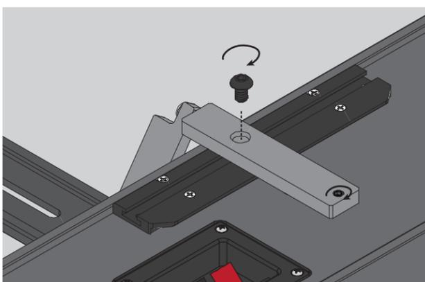
Slide speaker flush and centered with TV. Screw **Paddles** to T-nut in speaker's mount rails using **Short Button Head Screws**. Adjust speaker tilt using set screws in **Paddles**.
