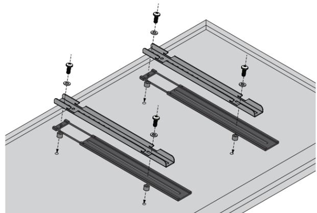
Affix **Adjustable Uprights** and **TV Mount Rails** with **M6 or M8 Screws** and **Washers**. Use **Spacers** as needed to ensure the **Adjustable Uprights** and **TV Mount Rails** are level.
