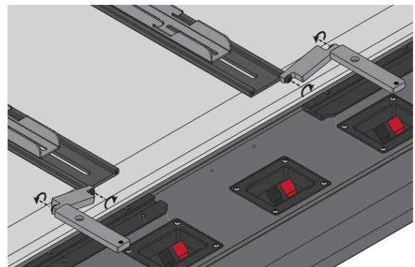
Position speaker so **Paddles** rest on speaker mount rails. Align T-nuts in mount rails with holes on **Paddles**. Tighten **Long Button Head Screws** with extra torque. (Mount rails and T-nuts come attached to speaker.)
