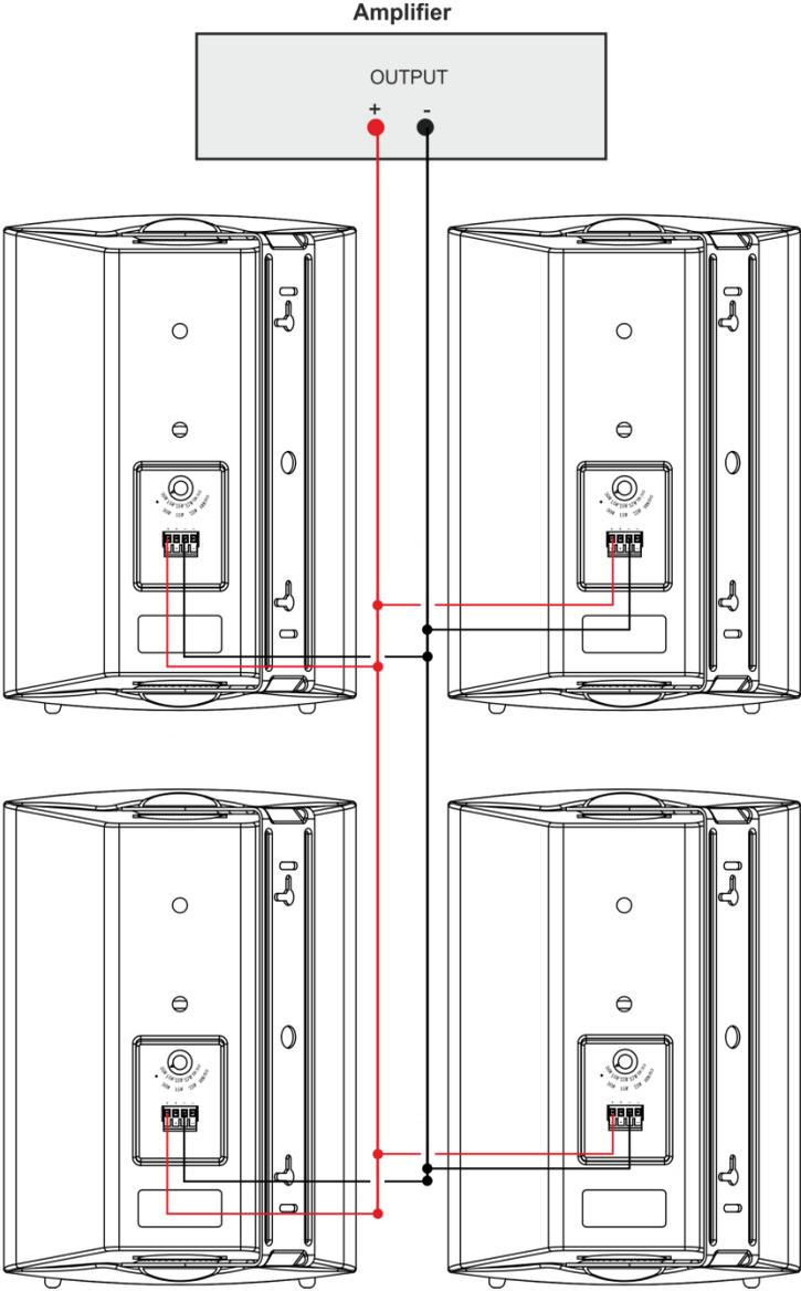
Figure 6: Square Layout Parallel Wiring
