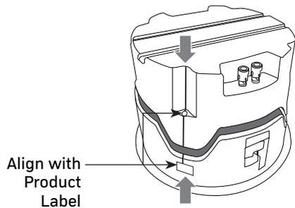
4. Secure enclosure to speaker using the screws provided.
