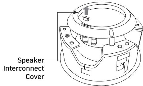
2. Attach the speaker to the appropriate enclosure before mounting.
