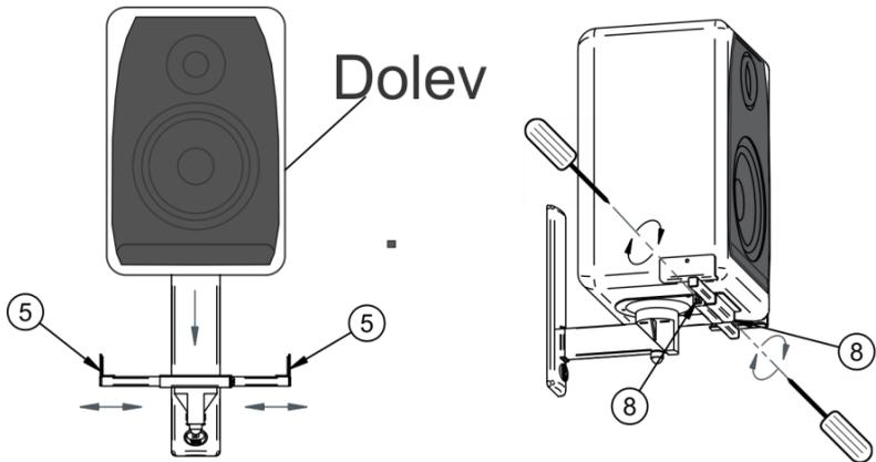
Figure 7: Attaching the Speaker to the Platform
