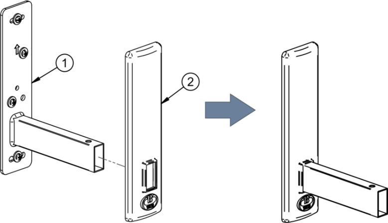
Figure 4: Sliding the Cover over the Wall Bracket
