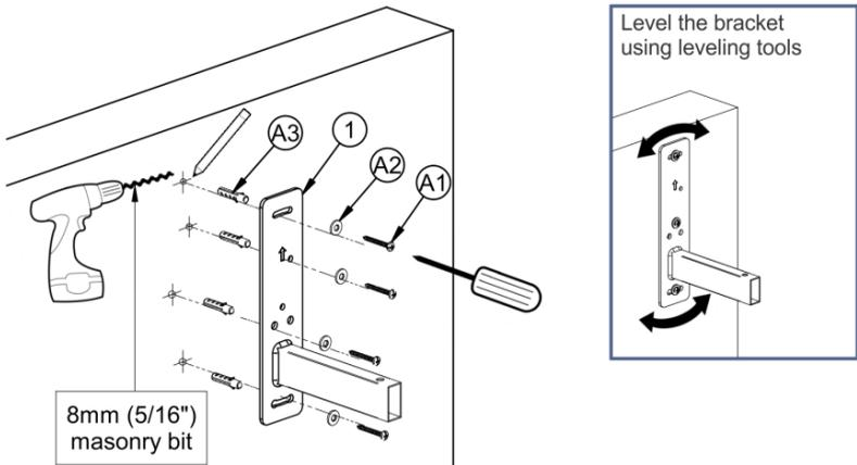
Figure 2: Attaching the Bracket to a Concrete Wall
