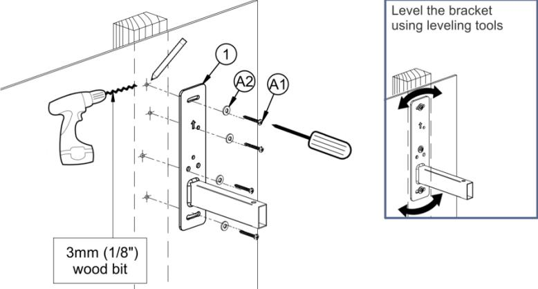
Figure 3: Attaching the Bracket to a Wood/Stud Wall
